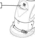
2. with a rubber tube, using the rubber cap (2) on the rear part of the solution tank.
