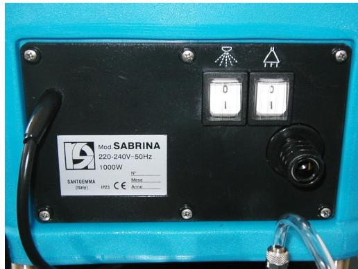
9. Switch on the air compressor, putting its switch in the position "I". The compressor switch is situated on the foam regulation control panel. In this way the compressor starts working and the pressure inside the air tank starts increasing. During this step, the arrow of the manometer indicating air pressure moves towards higher values.
