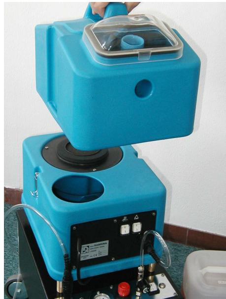
4. Put some fresh or warm water into the solution tank, through the circular hole, adding the product T-FOAM, in a ratio: 1 part of product and 4 parts of water.
